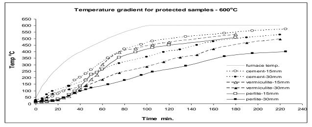
Fig.8: Temperature profile in protected unstrengthened specimens
