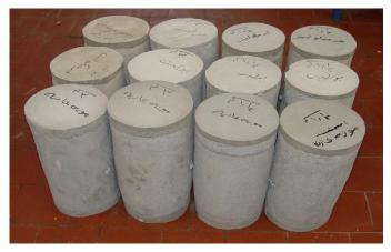
Fig.4: Concrete cylinders with different protection layers before subjecting to fire.
