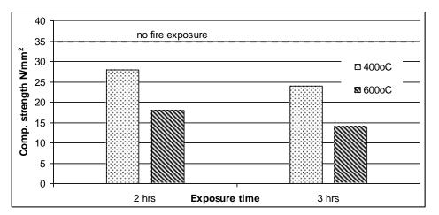
Fig 7: Effect of fire exposure on ultimate capacity of unprotected concrete specimens
