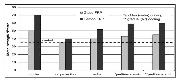
Fig 13: Effect of protection material on ultimate capacity of wrapped concrete specimens
