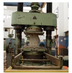
Fig.6: Experimental test set-up for testing the concrete cylinders.
