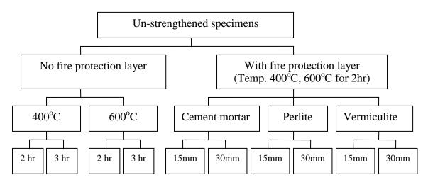
Fig.1 Experimental Program for unstrengthened specimens
