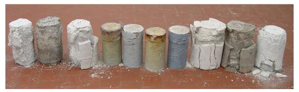
Fig. (11): FRP confined specimens subject to fire and axially loaded till failure
