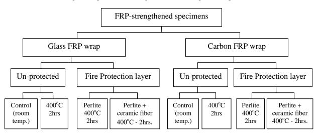
Fig.2 Experimental Program for FRP strengthened (confined) specimens
