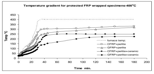
Fig.12: Temperature profile in protected FRP wrapped specimens
