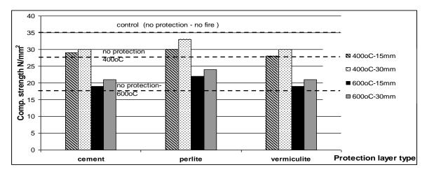
Fig 9: Effect of protection material and layer thickness on concrete strength
