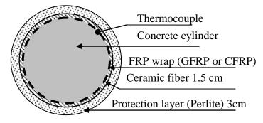
Fig.3 : Scheme of strengthening and protection layers applied to concrete cylinders.
